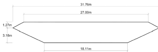
Figure 6: Shape of deck
